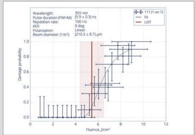
**Figure 2:** Real LIDT test data with the LIDT value shown by a red vertical line and a best fit 2-parameter Weibull distribution, showing that there is still some probability of damage below the LIDT value
