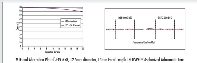
Aspherized Achromats are composed of glass optical lens elements bonded with a photosensitive polymer. The polymer is applied only on one face of the doublet and can be easily replicated in a short amount of time, providing the flexibility associated with typical multi-element components.
