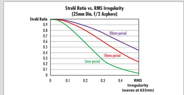
Figure 3: For a particular RMS surface irregularity, the more cosine periods over the aperture of the asphere, the lower the Strehl Ratio
