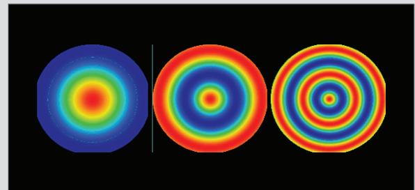
Figure 2: Radial cosine irregularity maps on a 25mm diameter  $f/2$  asphere surface. The cosine periods from left to right are 20mm, 10mm, and 5mm
