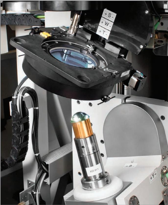
The QED Technologies® Aspheric Stitching Interferometer (ASI™) provides a full aperture map of the asphere being tested, and is capable of measuring complex aspheres with more than 600µm of aspheric departure. Edmund Optics® routinely measures complex asymmetric aspheric profiles and lenses with <math><0.5\mu\text{m}</math> surface figure requirements with the ASI™.
