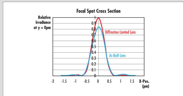
Figure 1: Irradiance cross section plot of the focal spot from a 25mm diameter  $f/2$  aspheric lens at 588nm. The Strehl Ratio of the as-built lens is 0.826, meeting the diffraction-limited criterion
